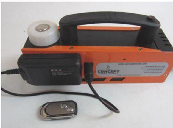
If you require the smoke button on the machine to latch on put the Slide Switch away from the reservoir.
