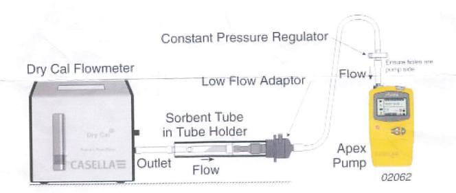
Please note the attachment may also be made to a dry flow meter or burette in the same manner. (Here a stopwatch will be required to measure the time to sample a specific volume.)
